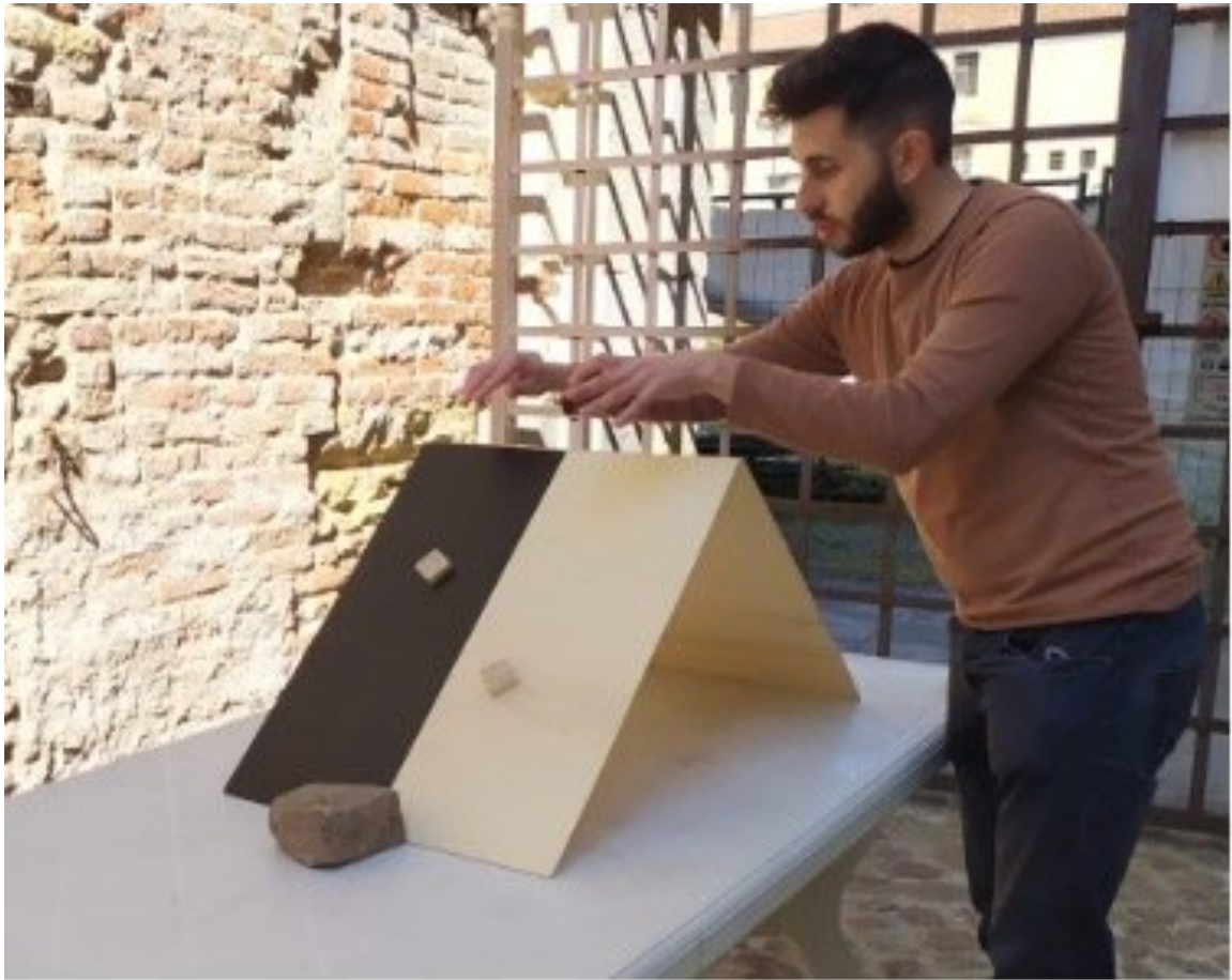
Figure 13 : Friction in action: one cube falls down the unpainted part of the inclined plane, while the other one on the painted part.
