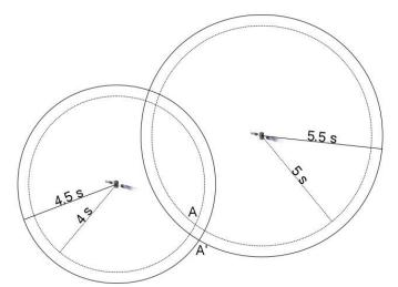
Figure 3: The same configuration as in Figure 2, but this time with a receiving clock running 0.5 s fast. Therefore, the signal transmission times are measured to be 0.5 s longer. This results in an intersection at A' instead of A.
