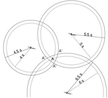
Figure 4: A third satellite is added, whose signal travel time is measured also measured wrongly. This leads to three intersections A' surrounding the true position A.
