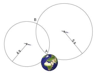
Figure 2: Configuration of two satellites. Position A on the Earth receives the signals after 4 and 5 seconds, respectively. The two signals intersect at points A and B. Since only A is on Earth, B can be discarded.
