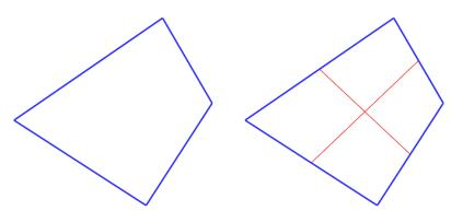
Figure 1: Illustration of how to approximate the centre of mass of an irregular tetragon. The shape is confined by four lines (left). After finding the bisectors of each line, the opposing bisectors are connected with a line (right). The intersection is an approximation for the centre of mass.
