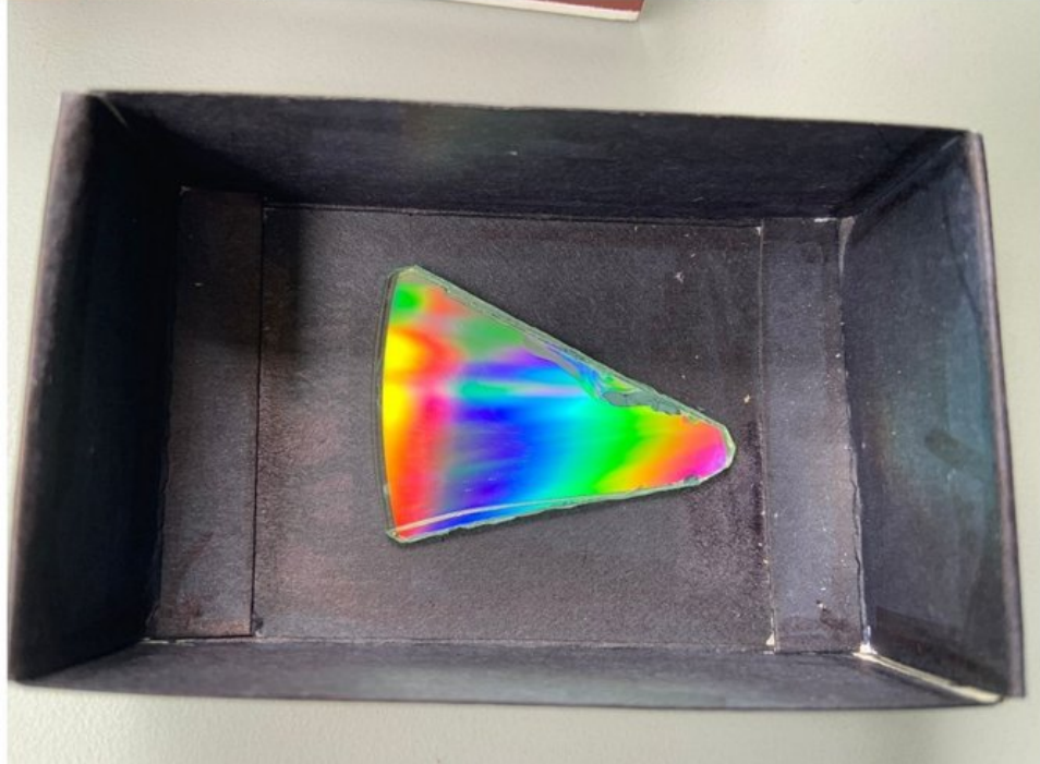
Figure 6: Gluing the piece of CD/DVD inside the matchbox.
