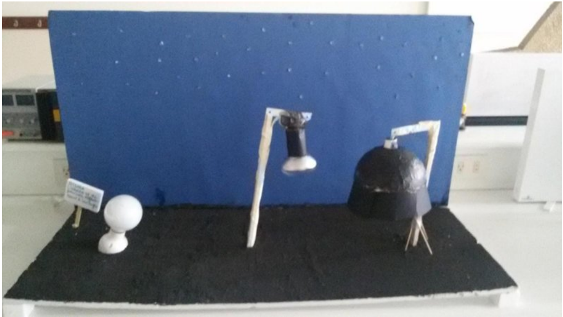
Image 1: three different light designs. From left to right, the first one is unshielded and fully directed towards the sky; the second one is partially shielded; the third one is well shielded and directed downwards.
