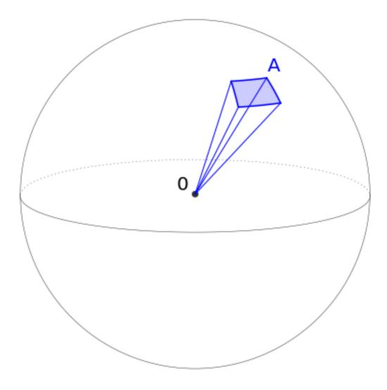
Since the object's light emission is spread evenly over the whole sphere, our detector will only receive a fraction A/(4 pi d  $^2$ ) of that emission; in other words, our detector will receive energy per second
